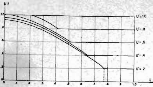
FIG. 7 OPTIMUM THICKNESS DISTRIBUTION OF FIXED-FREE VIBRATING ROD (B=U; j=1+U; \omega=\frac{\pi\sqrt{2}}{4}; U^0=1)
